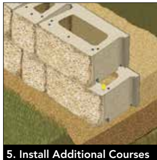
5. Install Additional Courses
